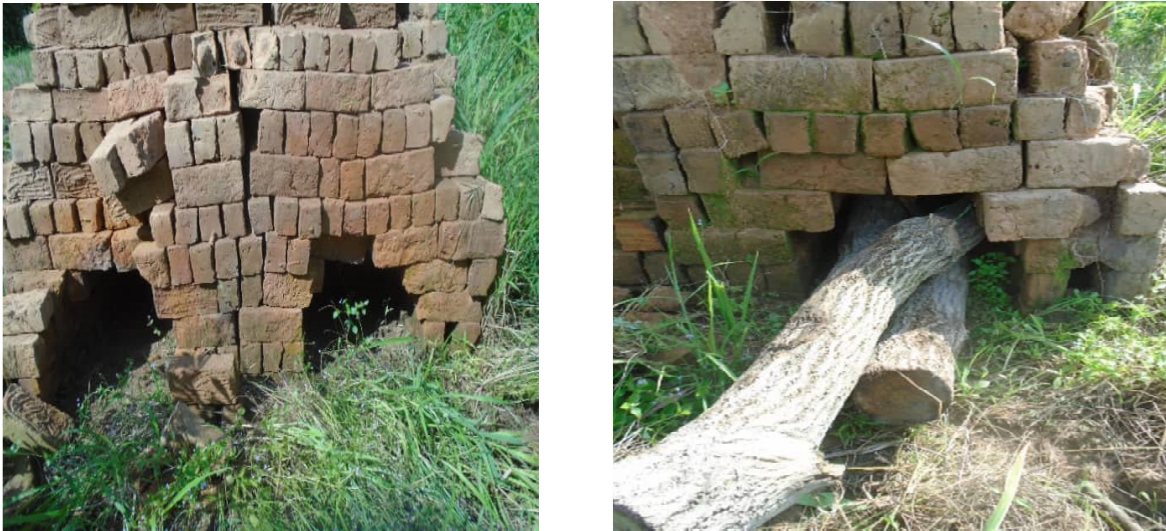
Figure 5: Loading Tunnels with Firewood
