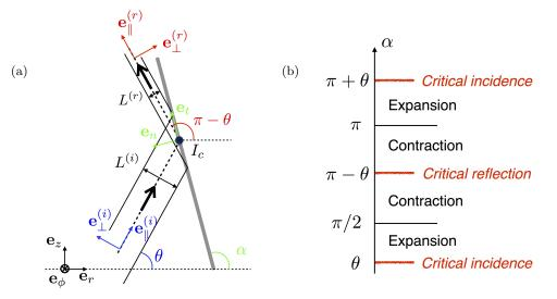
FIGURE 2. Reflection process. (a) Definition of the coordinate systems for  $0 < \theta < \alpha < \pi - \theta$ . Here the reflected beam is contracted because  $\pi/2 < \alpha < \pi - \theta$ . The relationships between the various coordinate systems are provided in appendix A. (b) Characteristic of the reflection process according to  $\alpha$  (assuming  $0 < \theta < \pi/2$ ).
