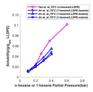
Figure 1. Solubility of n-hexane and 1-hexene in LLDPE (binary systems) at 70°C (data from Yao et al.<sup>[27]</sup> and Jin et al.<sup>[28]</sup>)
