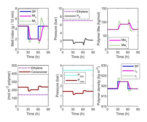
Figure 8. Grade transition in ethylene-1-butene: effect of the term  $w_5 \sum_{i=1}^{2} \frac{\Delta u_i}{u_i(t_0)}$  in the objective function ( $w_1 = 0.08$ ,  $w_2=1$ ,  $w_3=8$ ,  $w_4 = 19$  and  $w_5 = 10^4$ )
