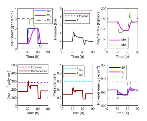
Figure 6. Grade transition in ethylene-1-hexene co-polymerization in presence of n-hexane: Tracking of the cumulative properties ( $w_1=w_3=w_5=0$ ;  $w_2=1$ ;  $w_4=4$ ), with constraints on the instantaneous properties ( $0.1<MI_i<3$  and  $910<\rho_i<935$ ).
