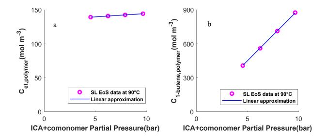
Figure 4. Concentrations in amorphous LLDPE obtained using SL EoS, Pseudo-quaternary system ethylene/(ICA+comonomer)/HDPE, at 90°C (after extrapolation of  $k_{ij}$ ) and 7 bar of ethylene: a) ethylene and b) comonomer 1-butene.
