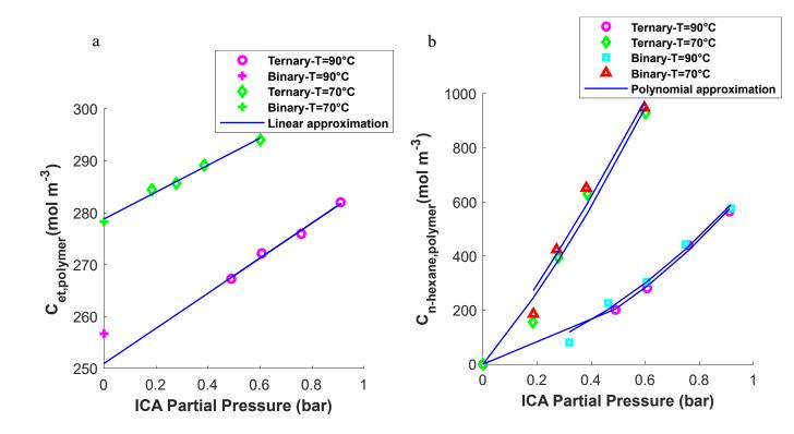
Figure 2. Ternary solubility data ethylene/n-hexane/LLDPE at 90°C and 70°C at 10 bar of ethylene (experimental data are taken for ternary systems from Yao et al.<sup>[31]</sup> and for binary systems from Yao et al.<sup>[27]</sup>): a) Concentration of ethylene in amorphous LLDPE as a function of the partial pressure of n-hexane, b) Concentration of n-hexane as a function of its partial pressure.
