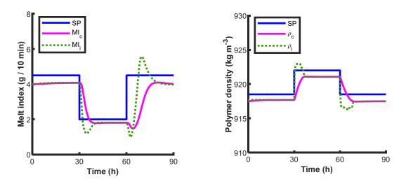
Figure 10. Influence of the thermodynamic model parameters on the process response, in ethylene and 1-butene copolymerization (Process parameters: A =1.98 mol m<sup>-3</sup> bar<sup>-1</sup>, E=180 mol m<sup>-3</sup>, Model parameters used for optimization: A =0.992 mol m<sup>-3</sup> bar<sup>-1</sup>, E=90.2 mol m<sup>-3</sup>)
