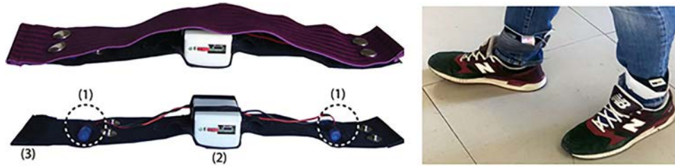
Fig. 1 The WEARHAP-PD device. The anklets are composed of two vibrating motors (1) attached to an elastic band (3). A Li-Ion battery and an Arduino board are in (2). When the device is engaged, its
