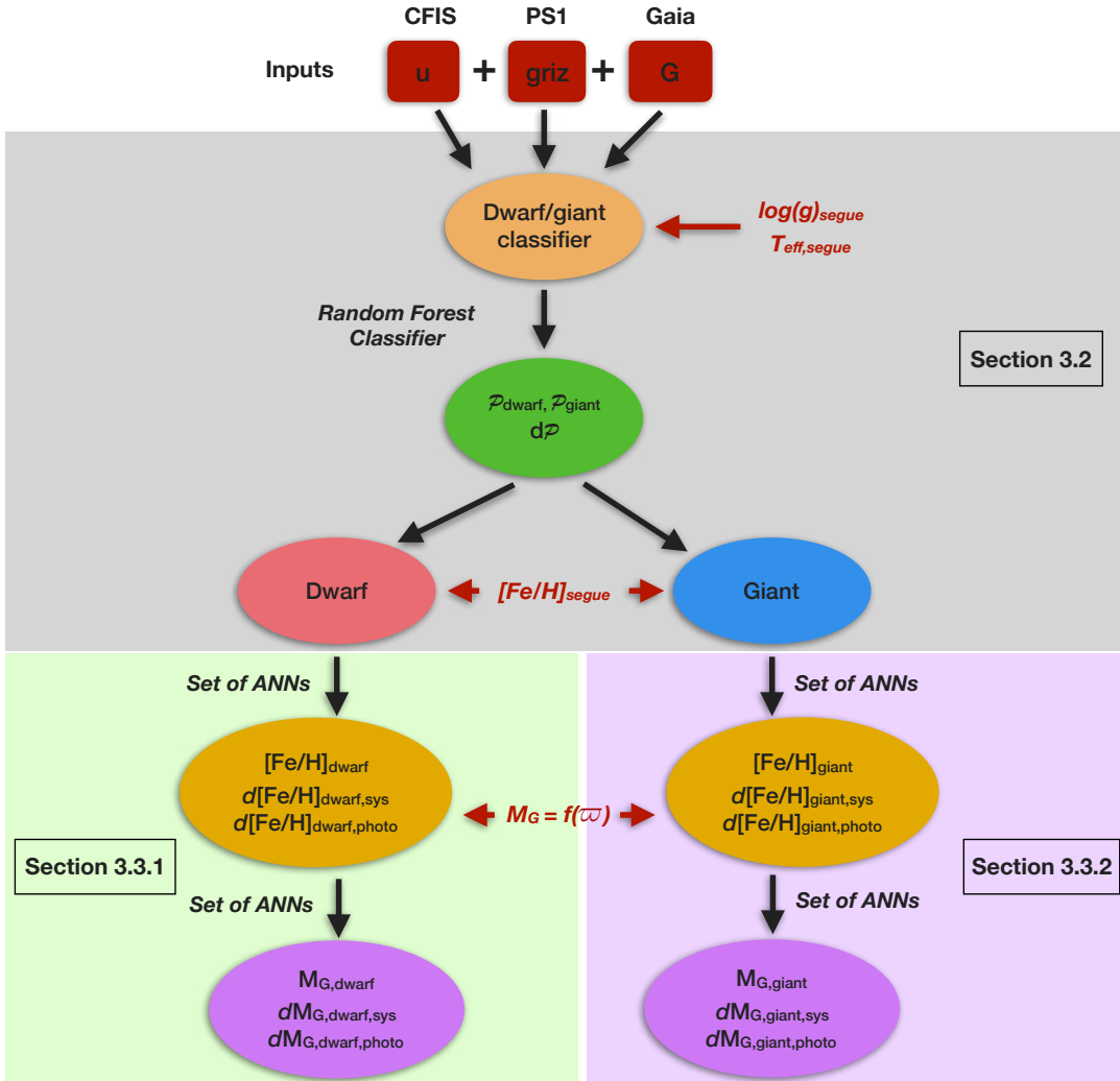
Figure 3. Schema of the algorithm described in Section 3. The input parameters are the photometric measurements from various surveys described in Section 2. Parameters in red are used for training. Dwarf - giant classification is done using a Random Forest Classifier . For each class, a set of Artificial Neural Networks (ANNs) is used to compute the photometric metallicity. Then, another set of ANNs is used to compute the absolute magnitude in the G -band, which provides the distances to the stars.
