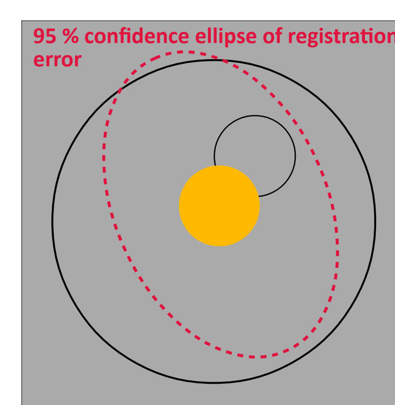
Figure 5 : Confidence ellipse constructed using registration error variance.
