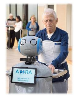
Astro is robot for mobility assistance and rehabilitation, used in hospitals or retirement homes. This robot was developed by Santa Anna University in Italy.
