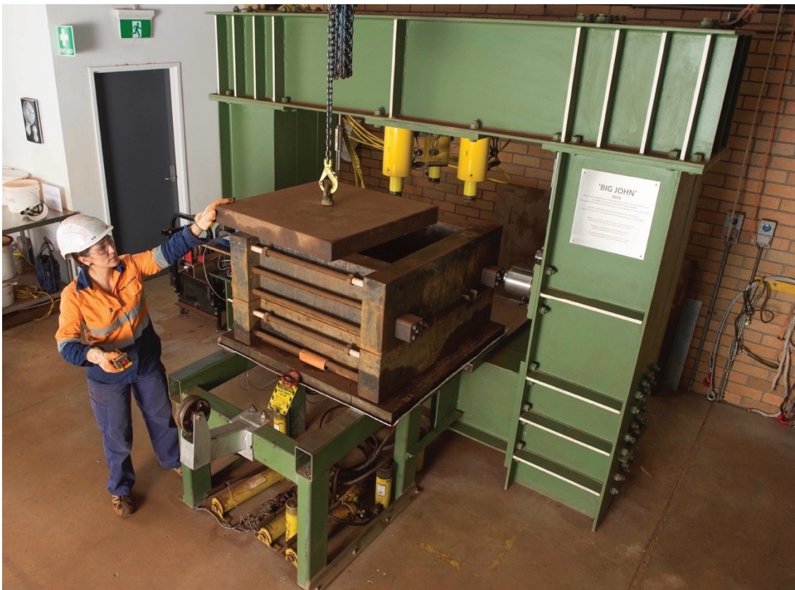
Figure 1 Overall view of the large direct shear apparatus with shear-box being positioned from the side using a mounting table, and the loading-plate being positioned using an overhead crane (Linero et al. 2019b)
