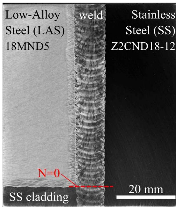
Figure 2: Optical macrograph of the dissimilar metal weld mock-up after post-weld heat treatment. Numbering of weld beads was started ( $N=0$ ) at the first bead in contact with LAS, as shown by the dotted line.
