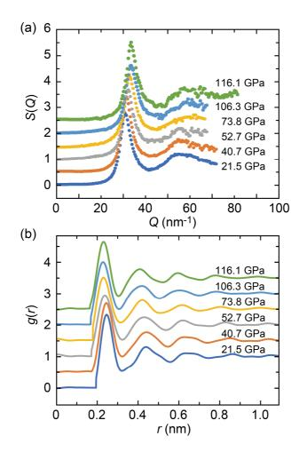
FIG. 1. Structural analyses of liquid iron at high pressures via in-situ XRD measurements. (a) Structure factor, S(Q), of liquid iron up to 116.1 GPa determined from XRD measurements in this study, showing peak shifts to larger Q values due to the compression of liquid iron. (b) Corresponding radial distribution functions, g(r), determined in this study. Vertical scales are offset for clarity for both S(Q) and g(r) plots.
