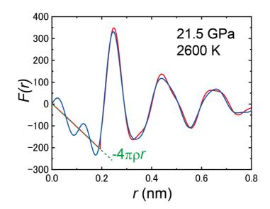
FIG. 2. Distribution function F(r) from run #1 calculated based on the present analytical method (red), in which the extension of S(Q) and parameters of s,  $a_N$ , and  $\rho$  are determined simultaneously, demonstrating that our new method successfully reduces the oscillations at  $r < r_{\min}$  and gives a precise liquid density from the slope. F(r) calculated without extension of S(Q) with assuming s = 1 is shown by the blue line for comparison.
