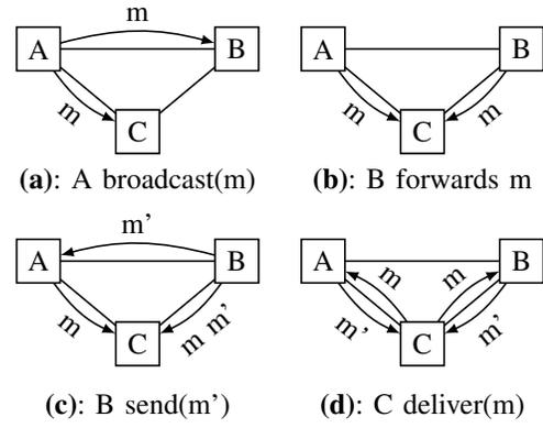
Fig. 1: Causal broadcast by FIFO forwarding [7]
