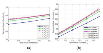
Fig. 5: Impact of equalization parameters on the EXIT chart performance: (a) MMSE filter lengths  $(N_1, N_2)$  (b) Number of  $3^{rd}$ order Volterra kernels,  $L_3$ .
