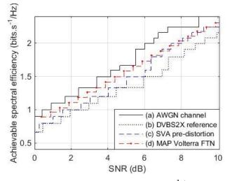
Fig. 9: Achievable Spectral Efficiency  $(bit.s^{-1}/Hz)$  Vs SNR (dB) - Range of low SNR
