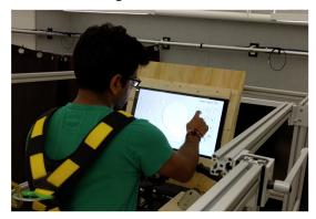
Figure 1: Experimental set up. Participants sat on a motion platform and made selections using a touchscreen or trackball. A transparent stencil (shown) was overlaid on the touchscreen.
