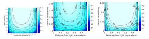
**Fig. 13** Computed velocity fields from Zhang and Chanson [37] for h = 0.175 m and Q = 0.0556 l/s (left), h = 0.085 m. and Q = 0.0261 l/s (center) and h = 0.155 m and Q = 0.0556 l/s (right)
