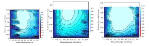
**Fig. 12** Experimental velocity fields from Wang et al. [34] for h = 0.175 m and Q = 0.0556 l/s (left), h = 0.085 m. and Q = 0.0261 l/s (center) and h = 0.155 m and Q = 0.0556 l/s (right)
