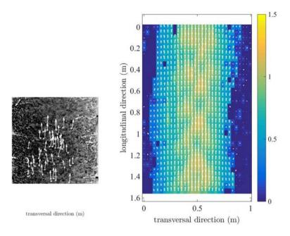
Fig.4 Recorded image and particule detected (left) and velocity field (m/s) for Q = 50 l/s and S = 1% (right)
