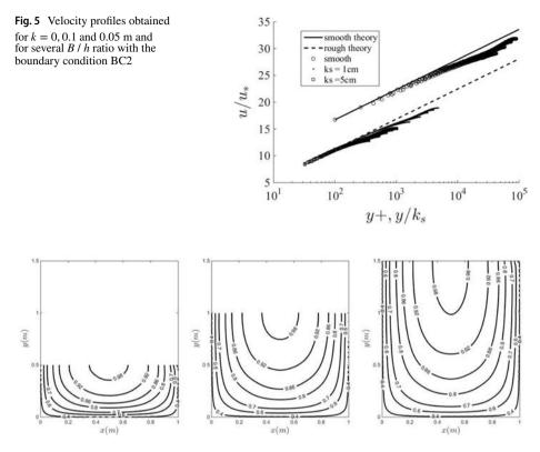
**Fig. 6** Isovels obtained for a rectangular channel with smooth condition ( $S_f = 0.001$ )
