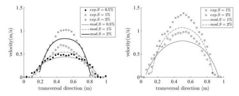
Fig. 9 Transverse profile of longitudinal velocity from experiments and proposed model for Q = 20 l/s (left) and Q = 50 l/s (right) at the free surface
