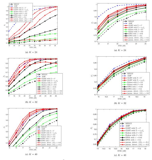
Fig. 3.  $P_d$  vs SNR in case of mismatched steering vector, for  $\cos^2\theta\approx 0.46$  and  $P_{fa}=10^{-4}$ .
