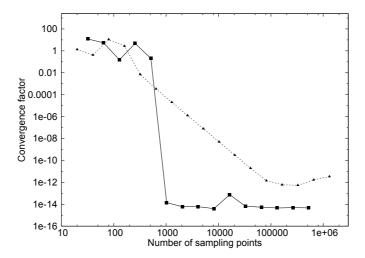
**Figure 3.** Convergence factor (33) for the FFT algorithm ( $\blacksquare$ ) and the Simpson algorithm ( $\blacktriangle$ ).
