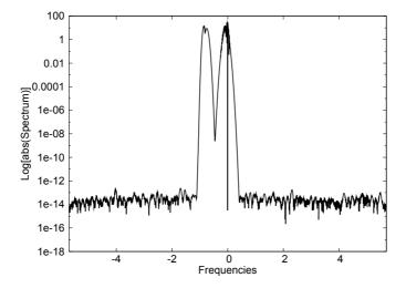
**Figure 2.** Absolute value of the spectrum of  $\tilde{f}(t)$  corresponding to (A.6) and (32). The function is given as a sample of N=2048 values equally distributed on the interval [0,T].
