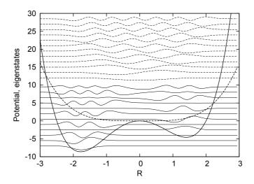
**Figure 5.** The two potential energy curves and some of the first unperturbed vibrational eigenstates of the first potential surface (full lines) and of the second one (dashed lines). The potentials are quartic polynomials defined as:  $\epsilon_1(R) = -5R^2 + 0.5R^3 + R^4$ ;  $\epsilon_2(R) = 0.2R^4$ .
