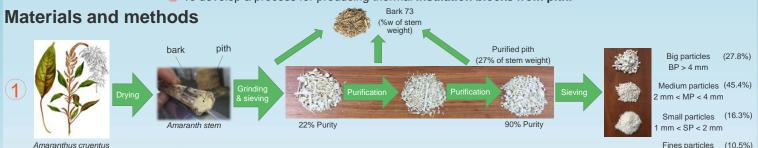
A Separation of bark and pith from the amaranth stem by a grinding, sieving and blowing (for pith purification) process.
