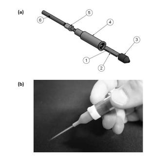
Fig. 4 Design of the piezo-plasma jet stylus (a) : (1) PT (2) electric connectors (3) stylus nozzle (4) stylus body (5) gas connector (6) gas tube. The piezo-plasma jet in operation (b) with a 1slm Ar gas flow
