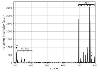
Fig. 5 Main emission lines of the plasma on a selected range of wavelengths
