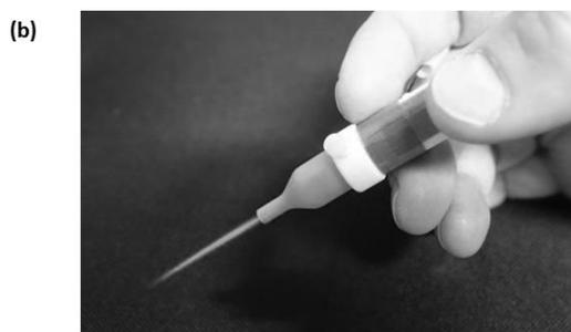
Fig. 4 Design of the piezo-plasma jet stylus (a) : (1) PT (2) electric connectors (3) stylus nozzle (4) stylus body (5) gas connector (6) gas tube. The piezo-plasma jet in operation (b) with a 1slm Ar gas flow
