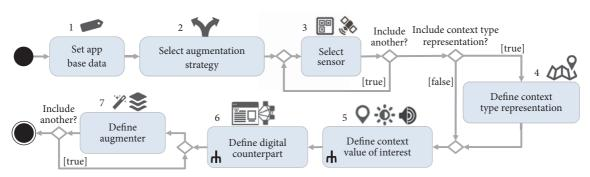
FIGURE 5: The supported process by the MoWA authoring tool.
