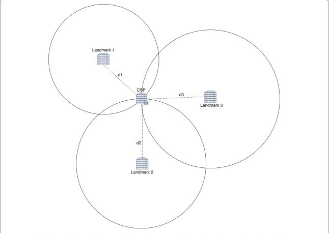
$\textbf{Fig. 7} \ \texttt{Example of perfect multilateration}. \ d_i \ \text{the estimated distance between} \ \textit{Landmark}_i \ \text{and CSP} \ \text{is the same as the real one}. \ \textit{Circles intersect at a point}$
