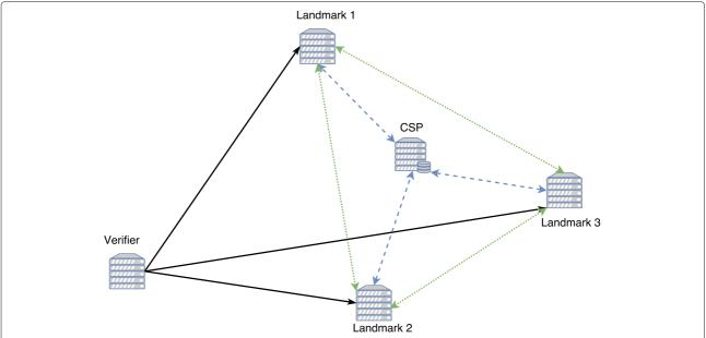
**Fig. 2** Structure of landmark-assisted verification approaches. Solid arrows represent verification monitoring data flow, dotted ones the inter-landmarks measurement data flow, and dashed ones the measurements data flow between CSP and landmarks
