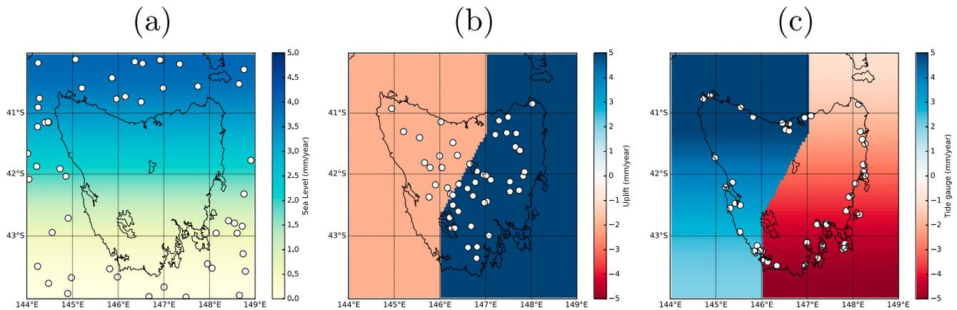
**Figure 9.** In (a) and (b) we show the true synthetic sea level rise and vertical land motion in mm/year. The derived tide gauge image is shown in (c). On each of the plots are shown the location of the randomly generated observations with small circles, that is, the location of sea level observations are shown in (a), GPS observations in (b), and tide gauges in (c).
