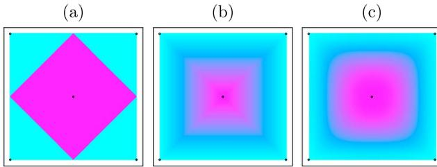
**Figure 1.** An example of the differences in each parameterization used in this study. Each of the parameterizations are defined with 5 points with a value of one at the center (0,0) and values of zero at the corners ( $\pm 1, \pm 1$ ). (a) Voronoi cell parameterization commonly used in trans-dimensional inversion, (b) linear Delaunay parameterization, and (c) cubic Clough-Tocher parameterization.
