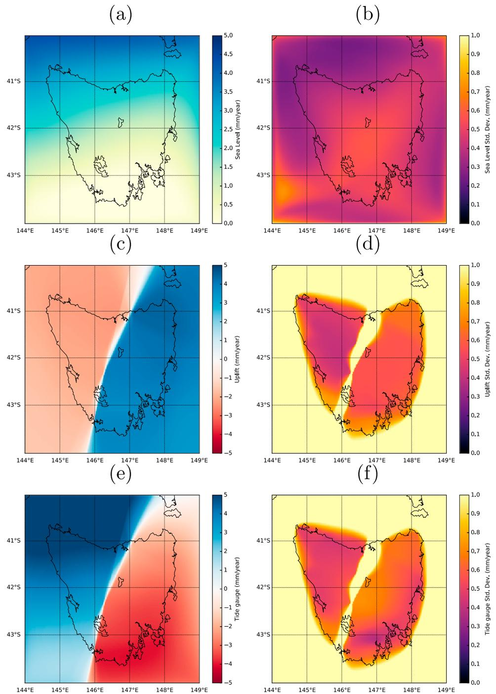
**Figure 11.** In (a), (c), and (e) we show the ensemble means of the rates of absolute sea level change (sea), vertical land motion (land), and relative sea level change (tide gauge) in mm/year, when using the Delaunay parameterization with linear interpolation for the sea model and Voronoi parameterization for the land. The maps of standard deviation are shown in (b), (d), and (f).
