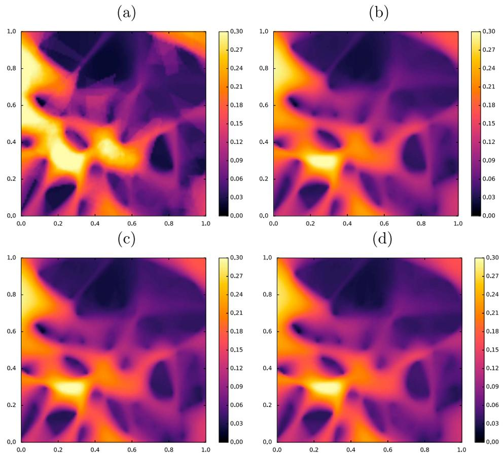
**Figure B1.** A comparison of the the standard deviation obtained from differently configure inversions. In (a) we invert a single chain; in (b) we use 28 independent chains as in the presented results but simulate 10 million steps; in (c) we use 56 chains; and in (d) we use 112 chains. In each case the estimated standard deviation is in agreement with results presented in Figure 3b.
