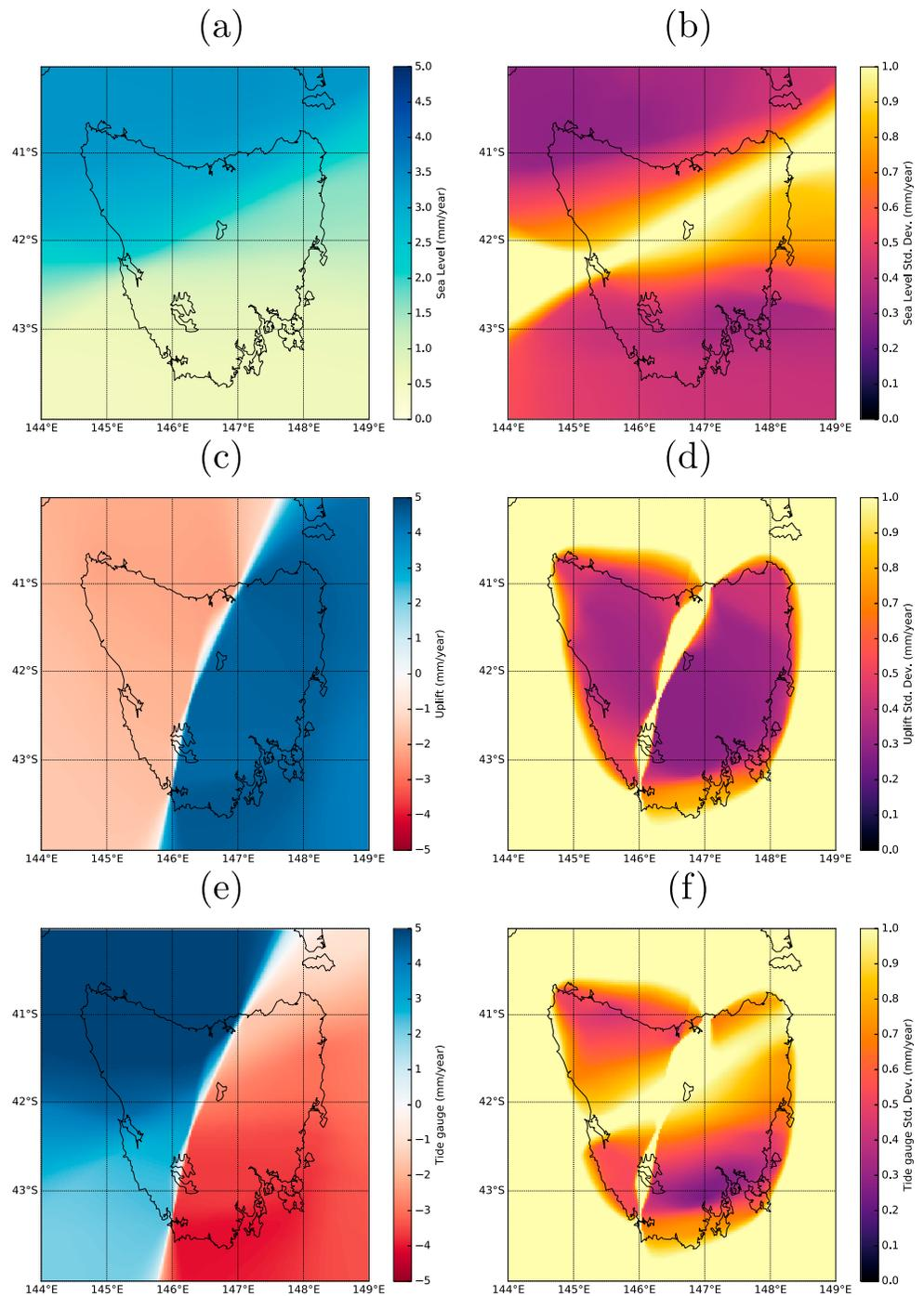
**Figure 10.** In (a), (c), and (e) we show the ensemble means of the rates of absolute sea level change (sea), vertical land motion (land), and relative sea level change (tide gauge) in mm/year, when using a Voronoi cell parameterization for both the sea and land model. The corresponding standard deviation maps are shown in (b), (d), and (f). Large uncertainties in the tide gauge standard deviation are caused by the Voronoi cell parameterization to represent the sea level.
