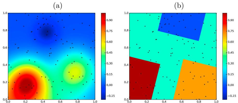
**Figure 2.** The true models used in the synthetic regression examples. (a) The true model is smooth and consists of a sum of four Gaussians, whereas (b) is a tessellated approximation of the same model with straight edges and discontinuities. The randomly located observation points are indicated with crosses.
