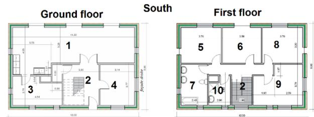
Figure 4: Sketches of ground and first floor of the building: kitchen coupled living-room (1), corridor (2), laundry (3), office (4), bedrooms (5, 6, 8, 9) and bathrooms (7,10)
