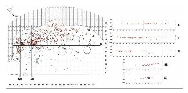
Figure 1. Site plan (left) and sections (right) of the transversal (60 and 58) and longitudinal (U, T, R) projections developed for the identification of sublevels a (red) and b (blue) of level P.
