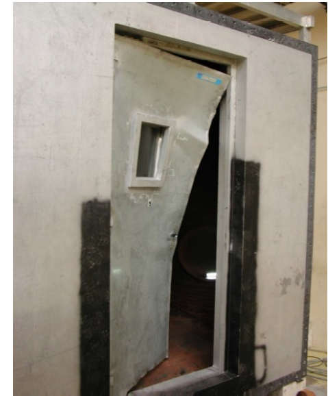
Test of mechanical behavior of a fire break door under a pressure stress in the STARMANIA facility
