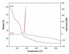
Fig. 1 TG-DTA curves of BCZT raw material.
