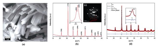
Fig. 2 (a) FE-SEM micrograph, (b) XRD, (c) SAED patterns, and (d) Rietveld refinement of BCZT powder calcined at 1000 °C/4 h.
