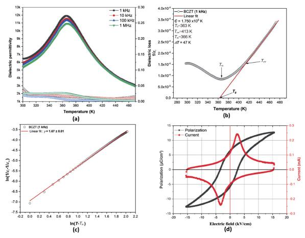
**Fig. 4** (a) Temperature-dependence of dielectric constant and dielectric loss, (b, c) plots of Curie–Weiss relation and modified Curie–Weiss law to determine slope ( $\gamma$ ), and (d) *P*–*E* and *I*–*E* plots of BCZT ceramics.
