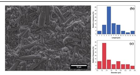
Fig. 3 (a) SEM micrograph and corresponding statistical distribution of (b) length and (c) diameter of BCZT ceramics sintered at 1250  $^{\circ}$ C/10 h.
