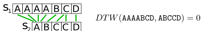
Fig. 8: DTW score equals to zero as successive identical elements in sequences are considered to be identical.
