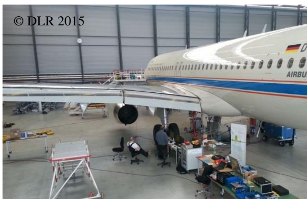
Figure 4: View of the overall GVT installation.
