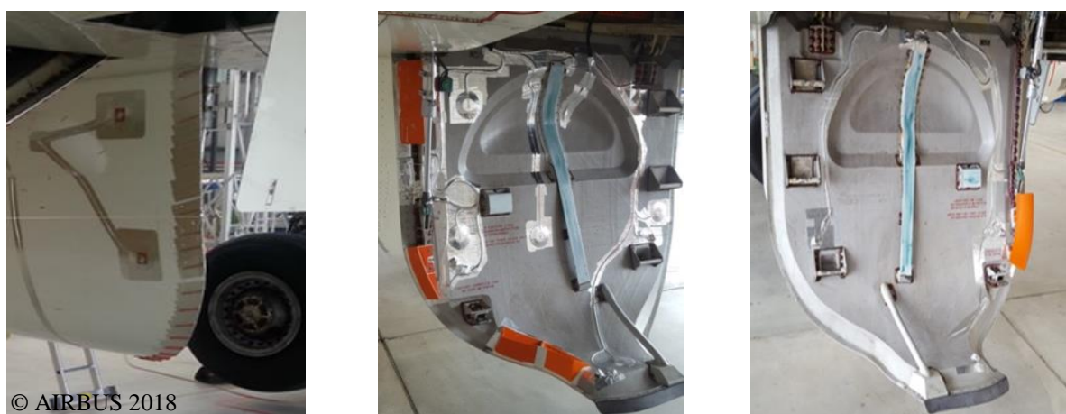
Figure 26: Main Landing Gear Doors device installation on Flight Test A/C (see [3]).
