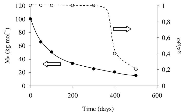
**Figure 7.11.** Variation in the number average molar mass  $M_n$ , and of the relative ultimate elongation  $\epsilon_R/\epsilon_{R0}$  in a polymer subjected to ageing by random chain scission at a rate of  $10^{-4}$  moles scissions per kg per day
