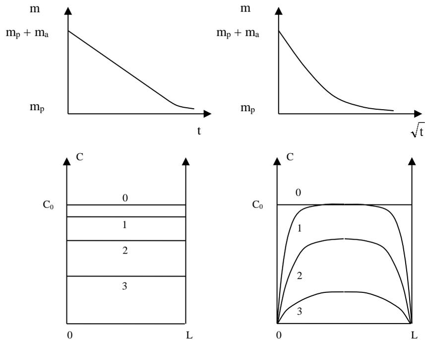
**Figure 7.7.** Migration controlled by evaporation (left) and by diffusion (right). Top: shape of the kinetic curves of mass evolution.  $m_p + m_a =$  polymer mass + additive mass ( $m_p =$  polymer mass). Bottom: additive concentration profile in the sample's thickness at different times:  $0 < t_1 < t_2 < t_3 < t_4$ .
