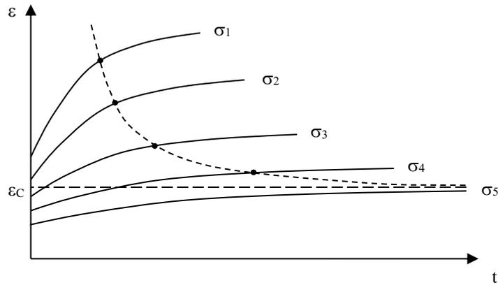
**Figure 7.4.** Shape of the creep curves in the presence of a solvent.  $\sigma_1 > \sigma_2 > \sigma_3 \dots$  etc. The black points represent onset of damage. The envelope of the points has a horizontal asymptote at  $\varepsilon = \varepsilon_c$
