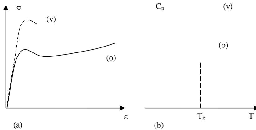
**Figure 7.3.** a) Shape of stress-strain curves from a new sample (o) and from a sample subjected to ageing under structural relaxation (v). b) shape of (DSC) thermograms from a new sample (o) and from a sample subjected to ageing under structural relaxation (v)
