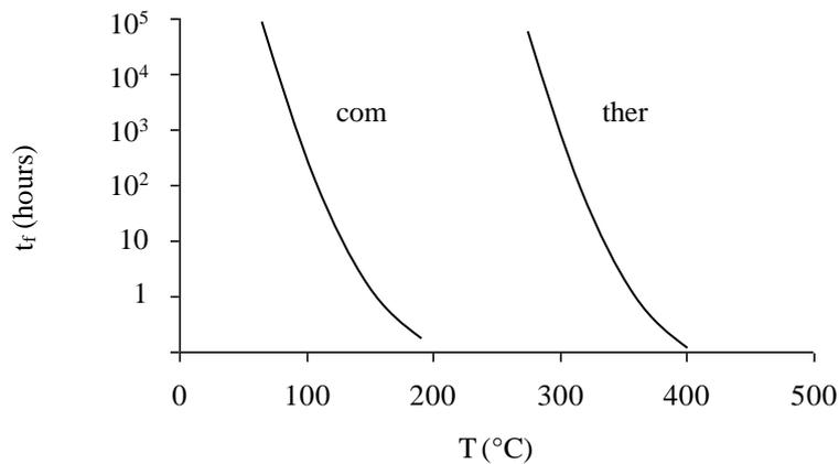
**Figure 7.19.** Lifetime (time to embrittlement) versus temperature. Curve shape for a commodity polymer (*com*) and for a thermostable polymer (*therm*).
