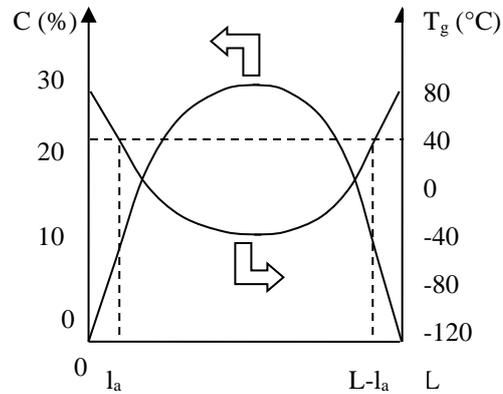
**Figure 7.8.** Presumed shape of the concentration profile in the plasticizer (mass fraction) and the local glass transition temperature in a plasticized PVC sample subjected to ageing at room temperature
