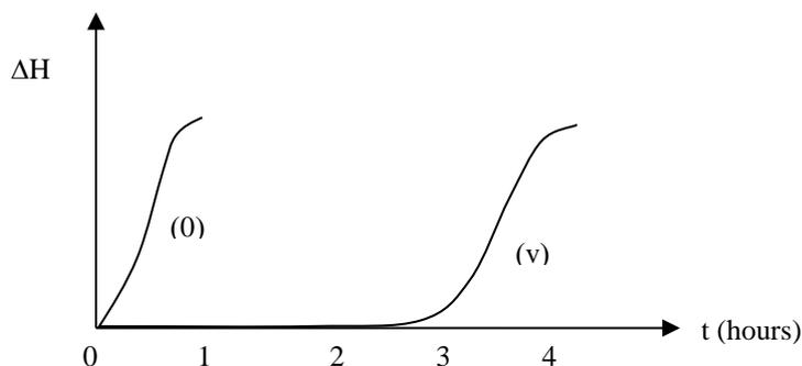
**Figure 7.17.** Shape of thermograms at 190°C (raise in temperature under nitrogen, oxygen is admitted in the cell when the thermal equilibrium has been reached): a non-stabilized polyethylene (0), the same polyethylene stabilized by 0.3% of a phenol-phosphite combination.
