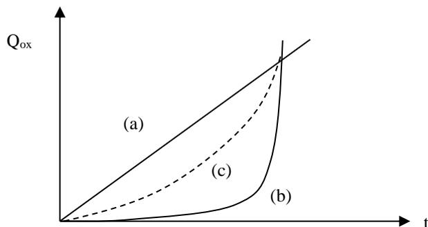
**Figure 7.16.** Shape of the kinetic curves of oxidation (a) for constant rate initiation (radiochemical ageing) (b) initiation by bimolecular decomposition ( $\delta = 2$ ) of hydroperoxides (thermal ageing). In cases of unimolecular initiation ( $\delta = 1$ ) of hydroperoxide (c) initial auto-acceleration is more progressive (some cases of photochemical ageing).
