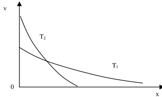
**Figure 7.13.** Diagram representing degradation profiles (thermo-oxidation) at two different temperatures:  $T_1 < T_2$  and at a sensitively equal total degradation rate
