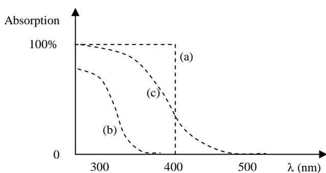
**Figure 7.22.** Absorption spectrum of UV absorbers: (a) ideal UV absorber; (b) UV absorber with limited protective power but colorless; (c) efficient UV absorber but yellow (it absorbs at  $\lambda > 400$  nm in violet)
