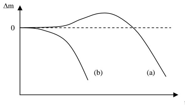
**Figure 7.18.** Shape of mass variations during thermal oxidation. (a) polymer with a relatively low initiation rate. Mass gain prevails during the induction period. Mass loss prevails after the mass gain has ended; (b) polymer with a relatively high initiation rate: mass loss prevails as exposure begins.
