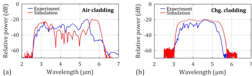
Fig. 2. Experimental (blue) and simulated (red) spectra measured out of the air cladded (a) and chalcogenide cladded (b) SiGe/Si waveguide with the same  $3.75 \times 2.7 \mu\text{m}^2$  core cross-section. The waveguides were pumped with pulses at  $4 \mu\text{m}$  and  $4.15 \mu\text{m}$  respectively, with 2.3 kW of coupled peak power.
