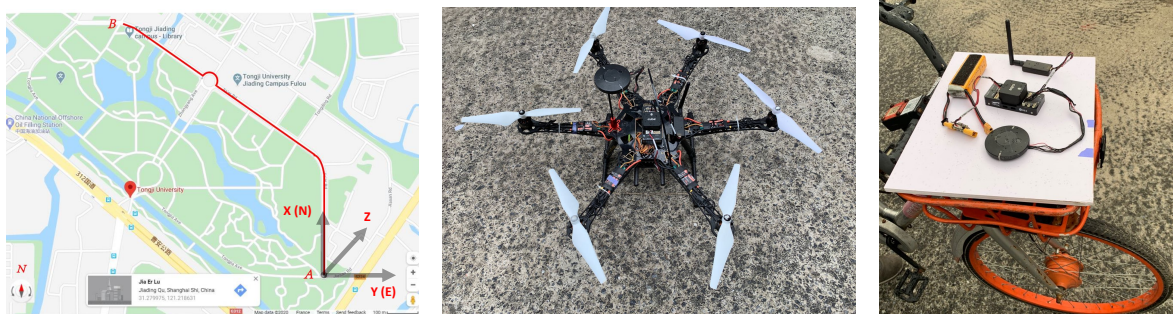
(a) Experiments path in Tongji University - Jiading Campus. (b) The UAV employed with a Pixhawk autopilot system. (c) The Pixhawk autopilot system deployed on a bicycle.
