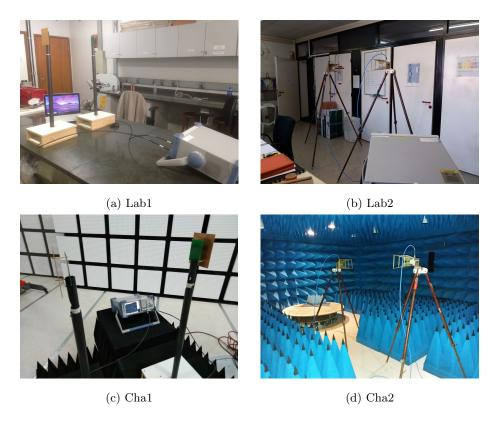
Figure 1: Test setups mounted for this investigation.
