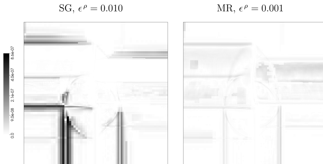
Figure 15: Lax–Liu Config. # 10: Local L_{1,AMR}^\rho -norm contribution |\rho_{i,j}^\ell - \rho_{i,j}^r| \Delta x_\ell \Delta y_\ell in gray scales for the SG and MR computations of Fig. 14 with WENO3 at final time t_{\text{end}} = 0.15 .
