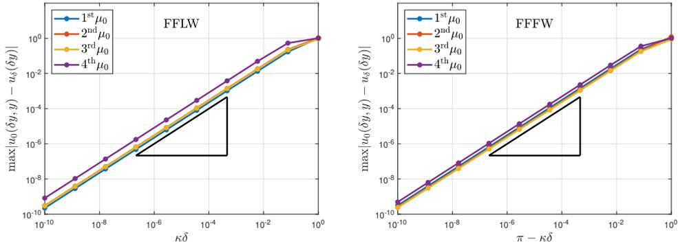
Figure 7: Loglog plot of the error between the exact (Bloch Floquet) and the homogenised fields for various values of  $\kappa\delta$  with  $\nu = 1$  and  $\nu = 0.5$ . (Left) FFLW. (Right) FFFW. The slope depicted by a black triangle denotes a  $O(\kappa\delta)$  (FFLW) or a  $O(\pi - \kappa\delta)$  (FFFW).
