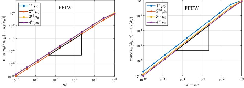
Figure 14: Loglog plot of the error between the exact (Bloch Floquet) and the homogenised fields for various values of  $\kappa\delta$  and for the same parameters used in Figure 11. (Left) FFLW. (Right) FFFW. The slope depicted by a black triangle denotes a  $O(\kappa\delta)$  (FFLW) or a  $O(\pi - \kappa\delta)$  (FFFW).
