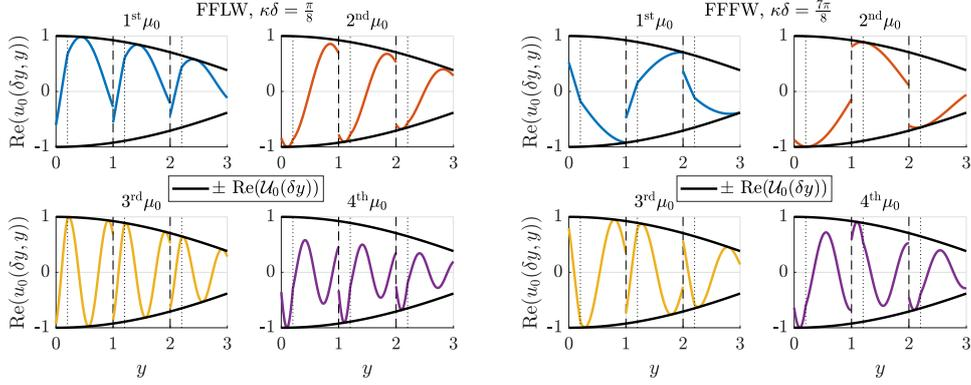
Figure 12: Real part of the field  $u_0(\delta y, y)$  corresponding the first four eigenvalues  $\mu_0$  along three unit cells for the bilayer case for the same parameters used in Figure 11. A dashed vertical line represents a boundary between two adjacent unit cells, while a dotted vertical line represents the location of the perfect interface between the two homogeneous materials. (Left) FFLW,  $\kappa\delta = \frac{\pi}{8}$ . (Right) FFFW,  $\kappa\delta = \frac{7\pi}{8}$ .
