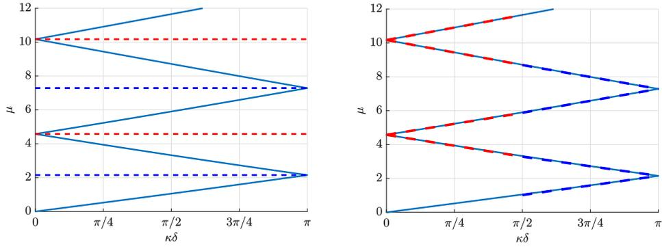
Figure 9: Dispersion diagram for the monolayer with  $\nu = 2$  and  $\kappa = 0.5$  corresponding to double eigenvalues. (Left) In red (resp. blue) dashed lines are the periodic (resp. antiperiodic) eigenvalues  $\mu_0$  calculated by finding the roots of (77). (Right) In red (resp. blue) dashed line are the periodic (resp. antiperiodic) resulting first-order approximations (73).
