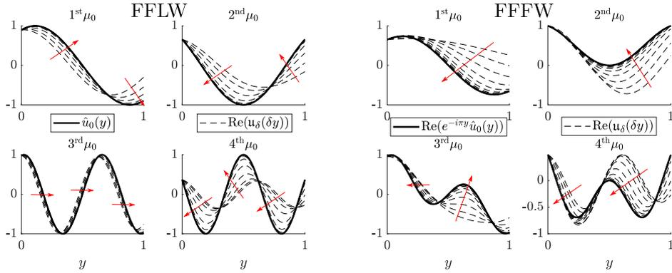
Figure 6: Illustration of the convergence of the method by comparing  $\hat{u}_0$  and  $u_\delta(\delta y)$  in the FFLW (left) and the FFFW (right) cases. We plotted  $u_\delta$  for 20 values of  $k\delta$  (FFLW) or  $\pi - \kappa\delta$  (FFFW) equidistributed in the log scale between  $10^{-5}$  and 1. The red arrows indicate how  $u_\delta(\delta y)$  is changing as  $\kappa\delta \rightarrow 0$  (FFLW) or  $(\pi - \kappa\delta) \rightarrow 0$  (FFFW).
