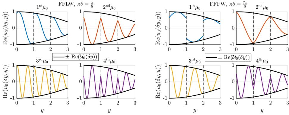
Figure 5: Real part of the zeroth-order approximation field  $u_0(\delta y, y)$  corresponding the first four eigenvalues  $\mu_0$  along three unit cells with  $\nu = 1$  and  $\nu = 0.5$ . A dashed vertical line represents the boundary between two adjacent unit cells. (Left) FFLW,  $\kappa\delta = \frac{\pi}{8}$ . (Right) FFFW,  $\kappa\delta = \frac{7\pi}{8}$ .
