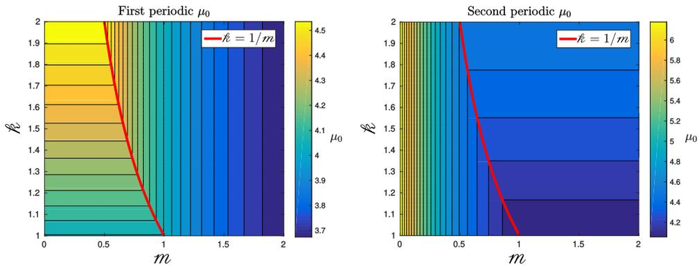
Figure 8: Filled contour plot of the first (left) and second (right) periodic eigenvalues  $\mu_0$  as  $\kappa$  and  $m$  vary. The thick red line represents the locus of double eigenvalues, while the thin black lines are isolines of  $\mu_0$ .
