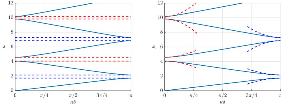
Figure 3: Dispersion diagram for the monolayer with  $\alpha = 1$  and  $\beta = 0.5$ . (Left) In red (resp. blue) dashed lines are the periodic (resp. antiperiodic) eigenvalues  $\mu_0$  calculated by finding the roots of (77). (Right) In red (resp. blue) dashed line are the periodic (resp. antiperiodic) resulting second-order approximations (55) using the computed values of  $T$ .
