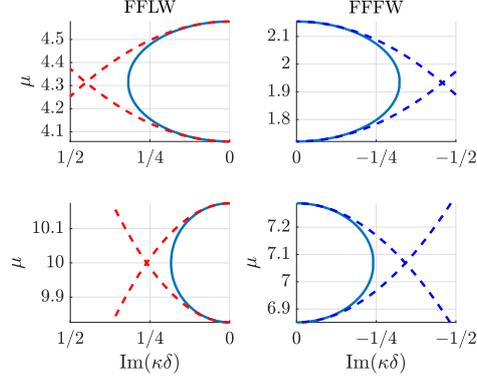
Figure 4: Imaginary part of  $\kappa\delta$  in the band gaps of the monolayer dispersion diagram for  $\nu = 1$  and  $\nu = 0.5$ . In red (resp. blue) dashed lines are the periodic (resp. antiperiodic) resulting second-order approximations (55) using the computed values of  $T$ , see also Figure 3 (right).
