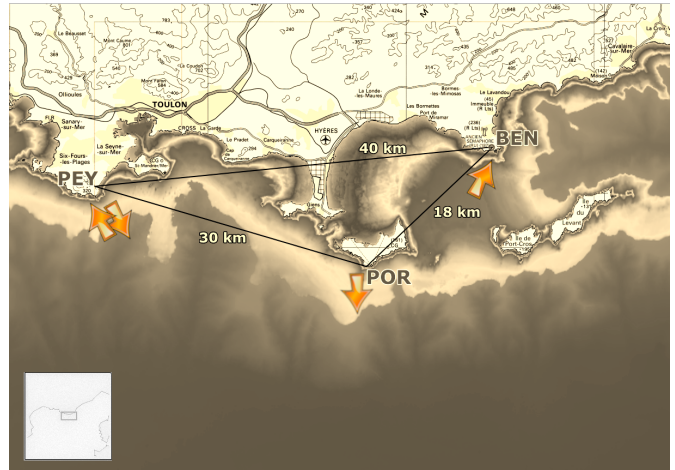
Fig. 2. The three HF radar sites in the region of Toulon: 1) Fort Peyras (TX/RX, “PEY”); 2) Cap Bénat (RX, “BEN”); 3) Porquerolles (TX, “POR”)
