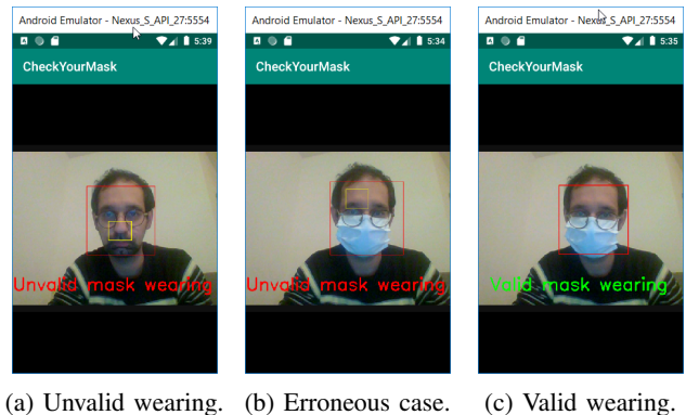
Fig. 3: Test of configurations with respect to Figure 1. The user wears glasses. The image background is homogeneous. A reusable white face protection mask made in tissue is used.
