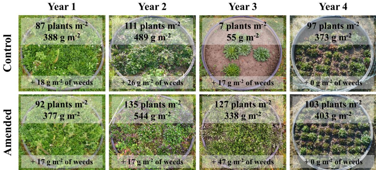
Fig. 1: Photos of the unamended lysimeter (“Control”) and the lysimeter amended with 5% biochar on the first 30 cm (“Amended”) taken in October of each year before harvest, with indication of the number of N. caeruleus individuals, the corresponding dry shoot biomass production, and the dry shoot biomass of weed plants per lysimeter (surface: 1 m 2 )
