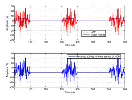
Fig. 1. Operating principle of NCP.
