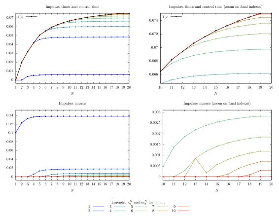
Figure 1: Illustration of the convergence of  $\underline{T}_N$ ,  $\tau_i^N$  and  $m_i^N$  as  $N \to \infty$  for the control system given in Section 4.1.
