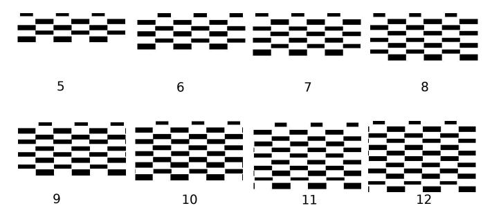
**Figure 2.** The best structures so far obtained on the Morpho problem for different numbers of layers. Three horizontal periods are actually represented here. The thicknesses of the blocks should be around 72 nm, the thickness of the air layers around 40 nm, the width of each block around 300 nm and the shift in the period should be either 0 or 300, or any other numbers as long as the difference is around 300 nm.
