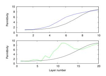
**Figure 3.** Refractive index profile obtained for an overall thickness of 700 nm and 10 (up) resp. 20 (below) layers. The curve in black represents a Gaussian profile, which is often presented as optimal for a continuous change of the refractive index in the literature. The index profiles shown here are clearly more efficient than a Gaussian profile (we have taken the standard deviation producing the lowest cost function and it proves difficult to beat).
