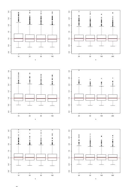
Figure 2: Boxplots of  $\hat{\theta}_p(x_0)/\theta_p(x_0)$  for Model 1 based on 500 replications of sample sizes n=500 (left column) and  $n=1\,000$  (right column) for p=1/(5n). From top to bottom we have  $x_0=3$ ,  $x_0=5$  and  $x_0=7$ . The values of k are taken as 2%, 5%, 10% and 20% of n.
