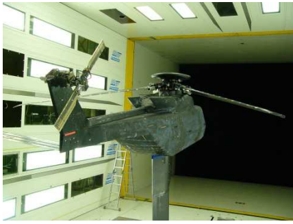
Figure 4. The GoAhead fully instrumented model in the DNW-LLF low speed wind-tunnel
