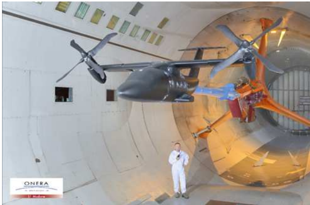
Figure 5. The European Nicetrip tilt-rotor model in the ONERA S1MA high speed wind-tunnel
