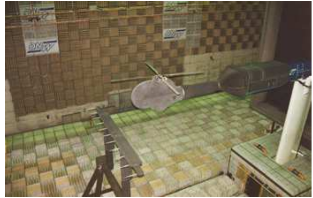
Figure 2. HART-II wind-tunnel tests in the DNW-LLF low speed wind-tunnel
