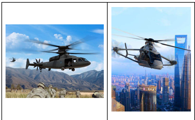
Figure 10. Two compounds concepts. Left: The Defiant from Sikorsky-Boeing. Right: The RACER from Airbus Helicopters
