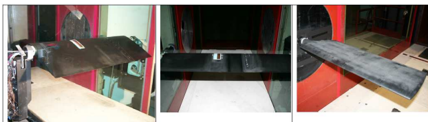
Figure 11. Dynamic stall OA209 oscillating wing models [32]
