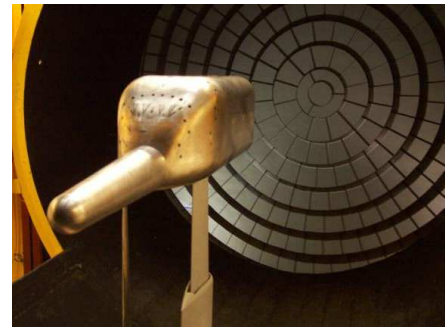
Figure 3. Active flow control on the ASF2 isolated fuselage in the ONERA L1 wind-tunnel
