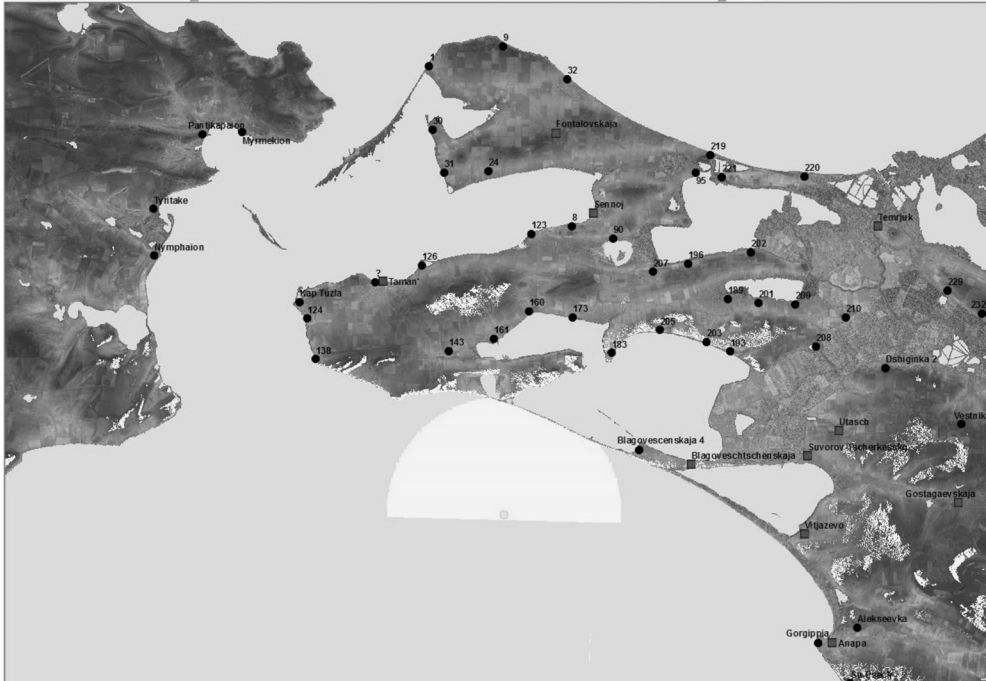
Fig. 9. Visibility study (including the Coracanda/Korokondamè/Korokondamitis ) from a ship in the Black Sea at the central point. Viewpoint is 10 m above sea level, the visible zones are represented in light grey. Based on SRTM 30 data, calculated by ARCGIS (© D. Kelterbaum)
