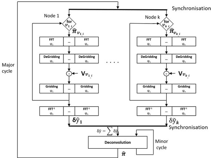
Fig. 3. Multi-node parallelization on independent frequency channels.
