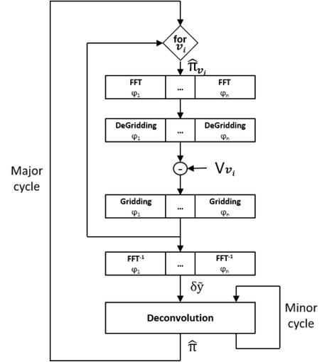
Fig. 1. DDFacet Single Node representation. Where  $\varphi$  is a facet,  $\pi$  is the sky model,  $g$  is the gridding result and  $\nu$  contains the visibilities for a set of frequencies  $\nu_i$ .
