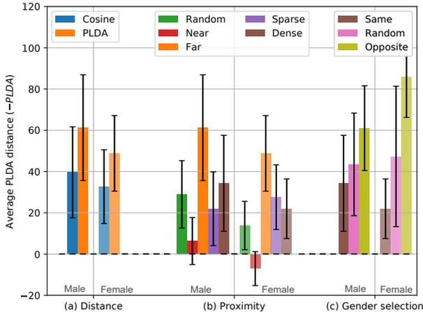
Figure 3: Average PLDA distance between original and anonymized  $x$ -vectors for different design choices. Comparison of: a) Distance with proximity as far and gender as same; b) Proximity with distance as PLDA and gender as same; c) Gender with distance as PLDA and proximity as dense. (Darker left bars: male speakers, Lighter right bars: female speakers)
