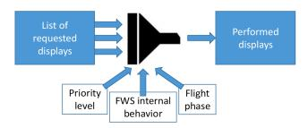
Figure 6: Principle for the display of the warnings
