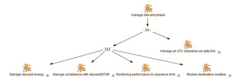
Fig. 5. "Manage descent phase" task model
