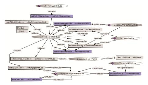
**Fig. 8.** ICO model of the ACI behavior for altitude management–Rectangles represent transitions (purple ones are enabled and light gray one are disabled); ellipses represent places; purple circles within places represent tokens (the number is the number of tokens in the place). (Color figure online)
