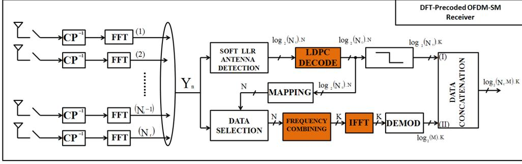
Fig. 2. Receiver structure of the proposed scheme.
