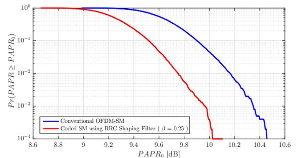
Fig. 3. PAPR comparison between Coded SM using RRC shaping filter and conventional OFDM-SM. Spatial multiplexing is done after FFT "precoding"
