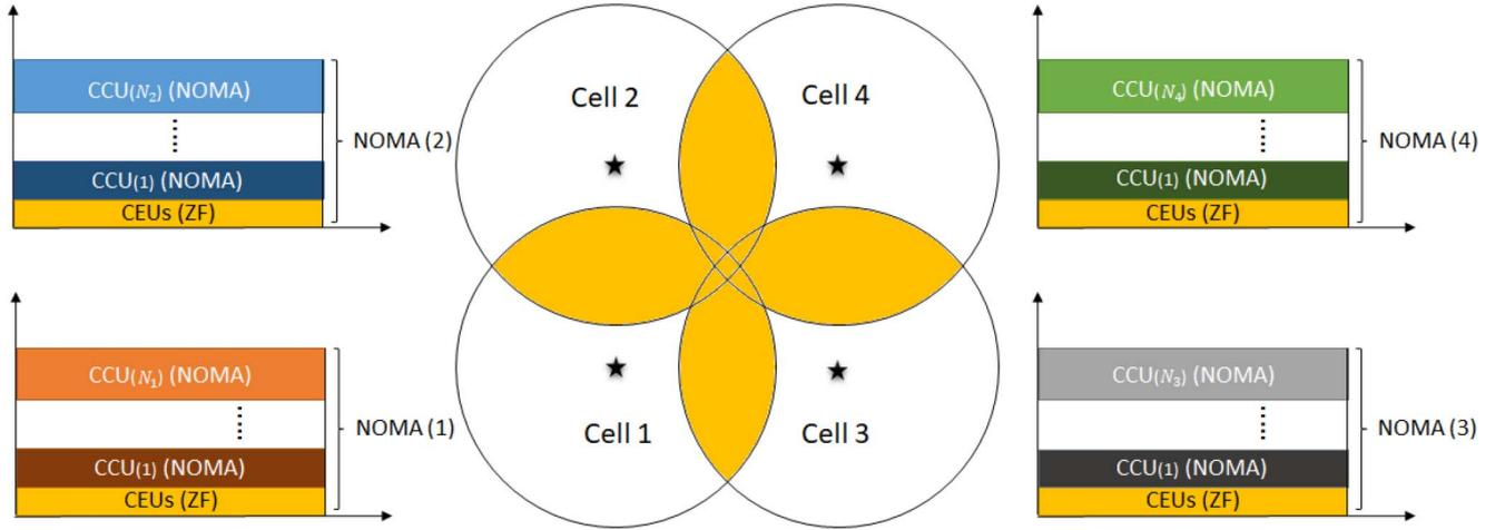
**FIGURE 2.** Illustration for the proposed hybrid NOMA-ZFP scheme for a 4-cell scenario. CEU locations correspond to the yellow colored areas, i.e., cell intersections. For instance,  $N_1$  denotes the number of CCUs in Cell 1.
