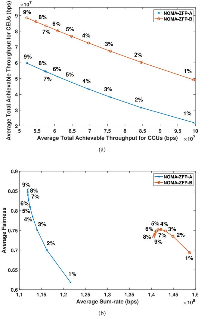
**FIGURE 10.** Comparison between (a) average achievable throughput for CCUs and CEUs; and (b) average network sum-rate and fairness for NOMA-ZFP-A and NOMA-ZFP-B schemes, for different percentages of power allocated to CEUs,  $a_{\text{CEU}}^2$ .
