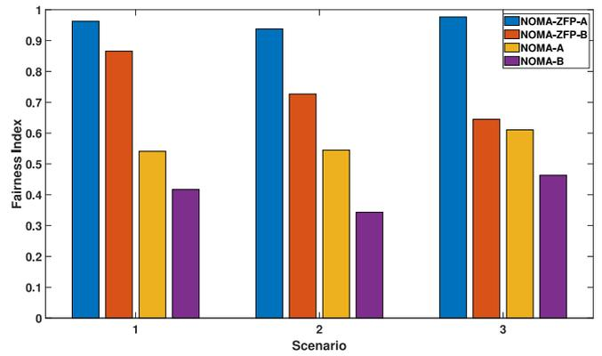
**FIGURE 5.** Network FI comparison for the considered MA schemes;  $P_O = 1.584$  W.
