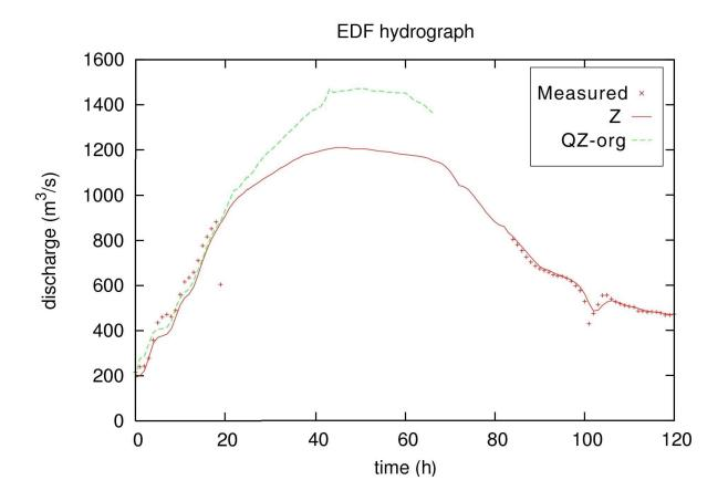
Fig. 10. Measured discharge hydrographs  $(m^3/s)$  at the middle gauge station EDF, and computed ones using the calibrated model (Manning is calibrated in 3 land classes, case b)). "Z": computed values with elevation imposed at downstream; "QZ-org": computed values with water stage hydrograph imposed at downstream.
