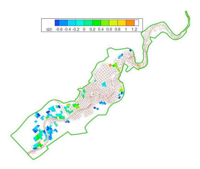
Fig. 9. Difference of water depth (m) at image instant (6:00, Feb 28th, 1997) between observations and computed values using the calibrated model (Manning is calibrated in 3 land classes, case b)).
