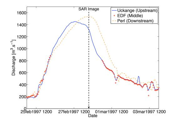
Fig. 2. Recorded hydrographs during the flood event at 3 different locations
