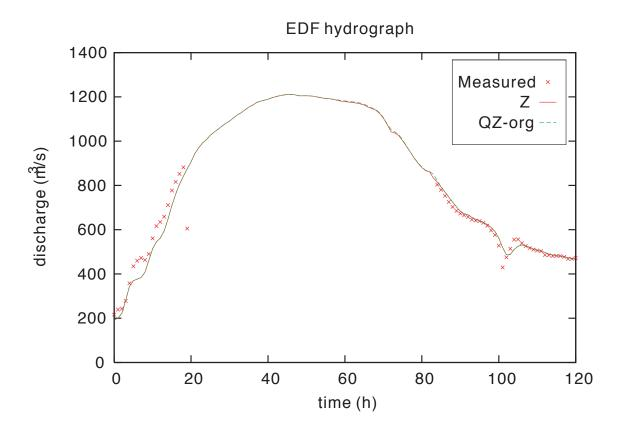
Fig. 5. Preliminary forward run. Comparison of discharge  $(m^3/s)$  at the middle gauge station EDF: measured, computed with elevation imposed at downstream ("Z"), computed with water stage hydrograph imposed at downstream ("QZ-org").
